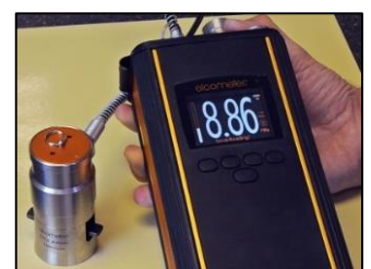
Fig. 1 : Schematic Diagram - Source Elcometer (left) - 510 Control Module and Traction Head - Source Elcometer (right)
